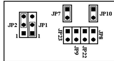
Figure 3: Jumper Configuration for UART0 as a DCE Device
