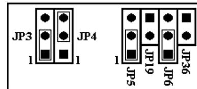
Figure 4: Jumper Configuration for UART1 as a DTE Device
