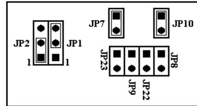
Figure 2: Jumper Configuration for UART0 as a DTE Device
