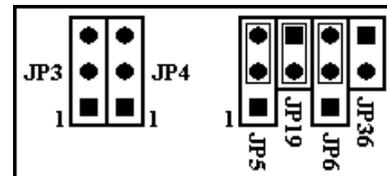
Figure 6: Jumper Configuration for UART1 for RS-485 communication
