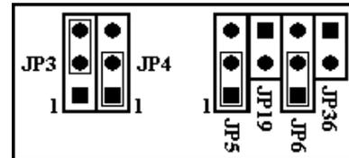
Figure 5: Jumper Configuration for UART1 as a DCE Device
